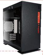
**Opening the Chassis** Please remove by pressing the handle on top of tempered glass side panel.
